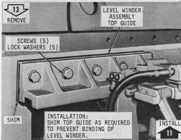
VIEW M. LEVEL WINDER ASSEMBLY TOP GUIDE.
