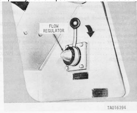
Figure 1-21. Flow regulator (adjustable)—installed view.
